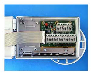
The terminal compartment is located in the bottom half of the 5202 housing. Depress the clip located on the right hand side and lift the cover to open the unit. The tension-spring terminals accept wire up to 18 gauge. All wires should be routed through the rubber grommets and strain relief clamps.
