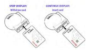
Withdrawing the card will stop the sequence at the current display, reinserting the card will restart the sequence. If the card is not reinserted, the LCD will switch back to the standard display in 24-hours.
