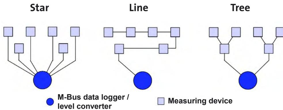
Star: All measuring instruments are wired directly to the central point. In the case of an error, the measuring instrument can be switched on or off to localize the defect.
