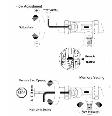
The memory stop allows return to previous flow rate setting after Flowguard has been used as a stop valve. (Totally closed flow)
