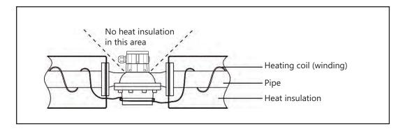
The permitted temperature ranges for the flow meter must be observed.
